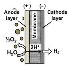
Figure 6 Cross-sectional view of PEM electrolysers
