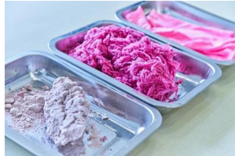
Cellulose powder and PET fibre separated by Hydrothermal treatment
