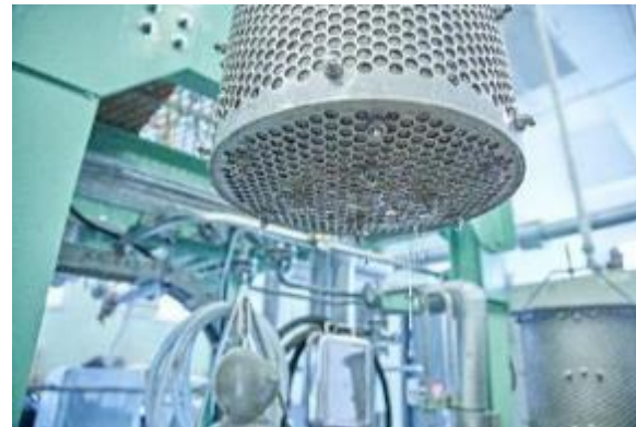
Filtration process of Hydrothermal Treatment
