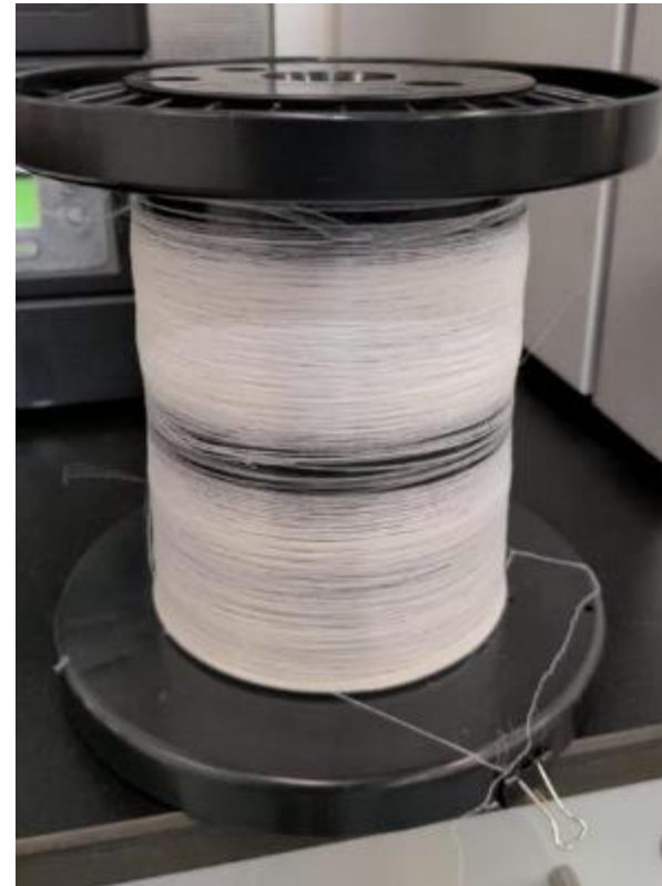
Finished fibre – mixing recovered cellulose powder with high DP cellulose and nanocellulose
